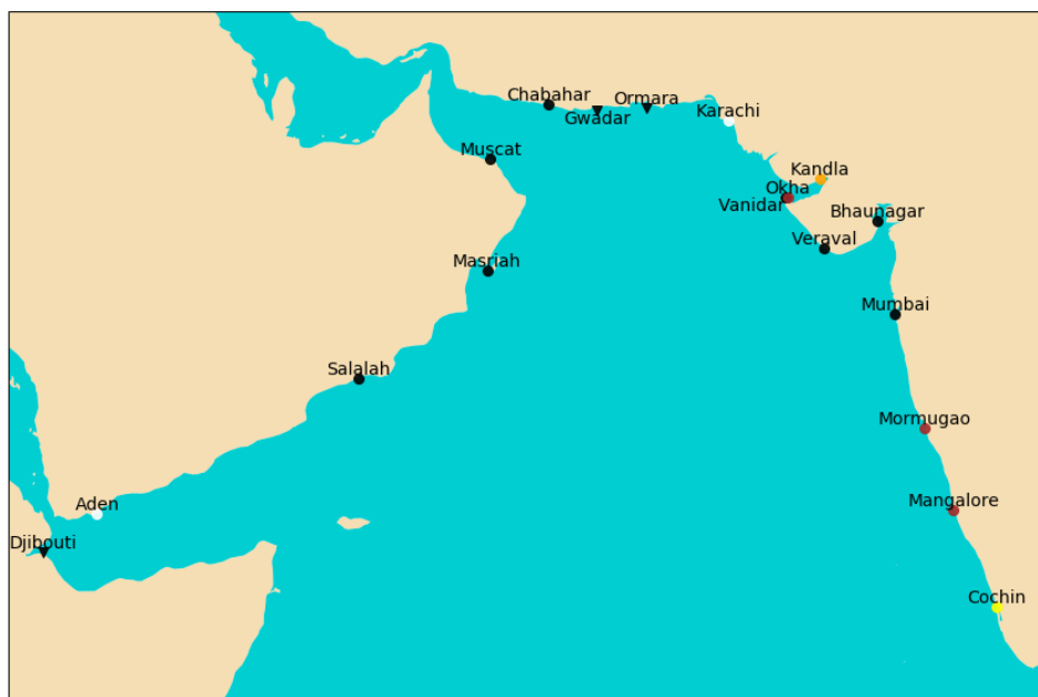
Figure A1.1a: Location of the 18 tide gauge stations for Arabian Sea. Time series length of more than: 100 years (white), 75 years (yellow), 50 years (orange), more 30 years (brown). Less than 30 years (black). Adapted from https://www.psmsl.org , Data Explorer.
