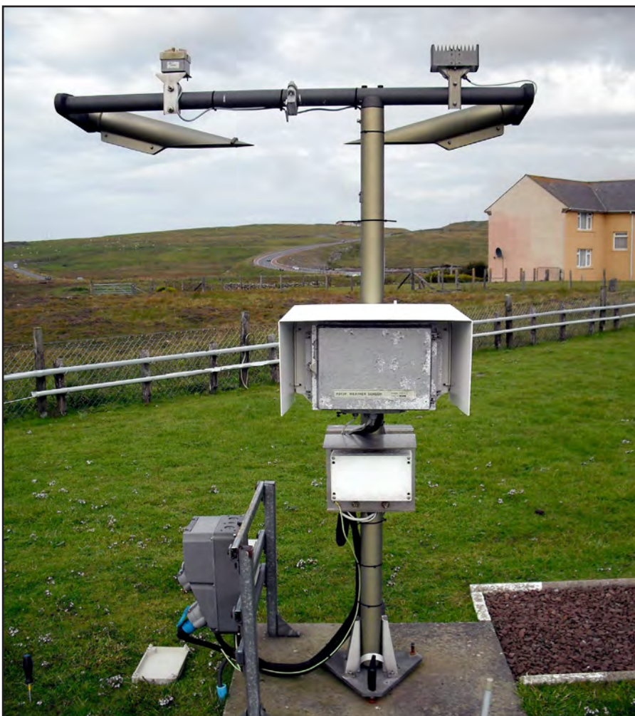
Figure 22. Present weather sensor.
