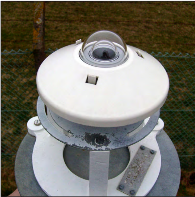
Figure 24. Pyranometer for measuring global radiation.
