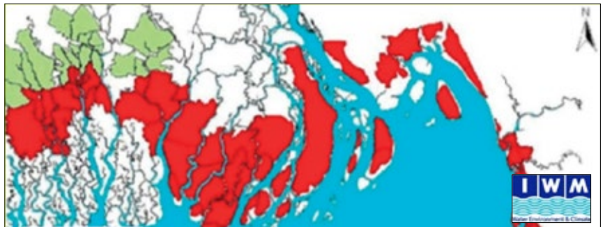
Figure 3. IWM study showing in red the 33 sea-facing and 26 interior-facing polders likely to be overtopped by 2050 based on global sea level projections.
