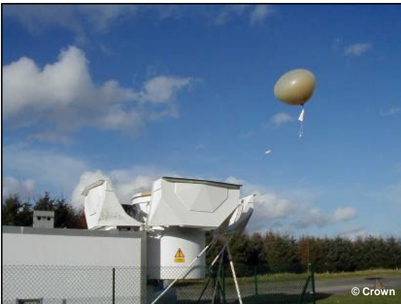
Figure 1. Vaisala AS12 autosonde releasing a balloon-borne radiosonde.
