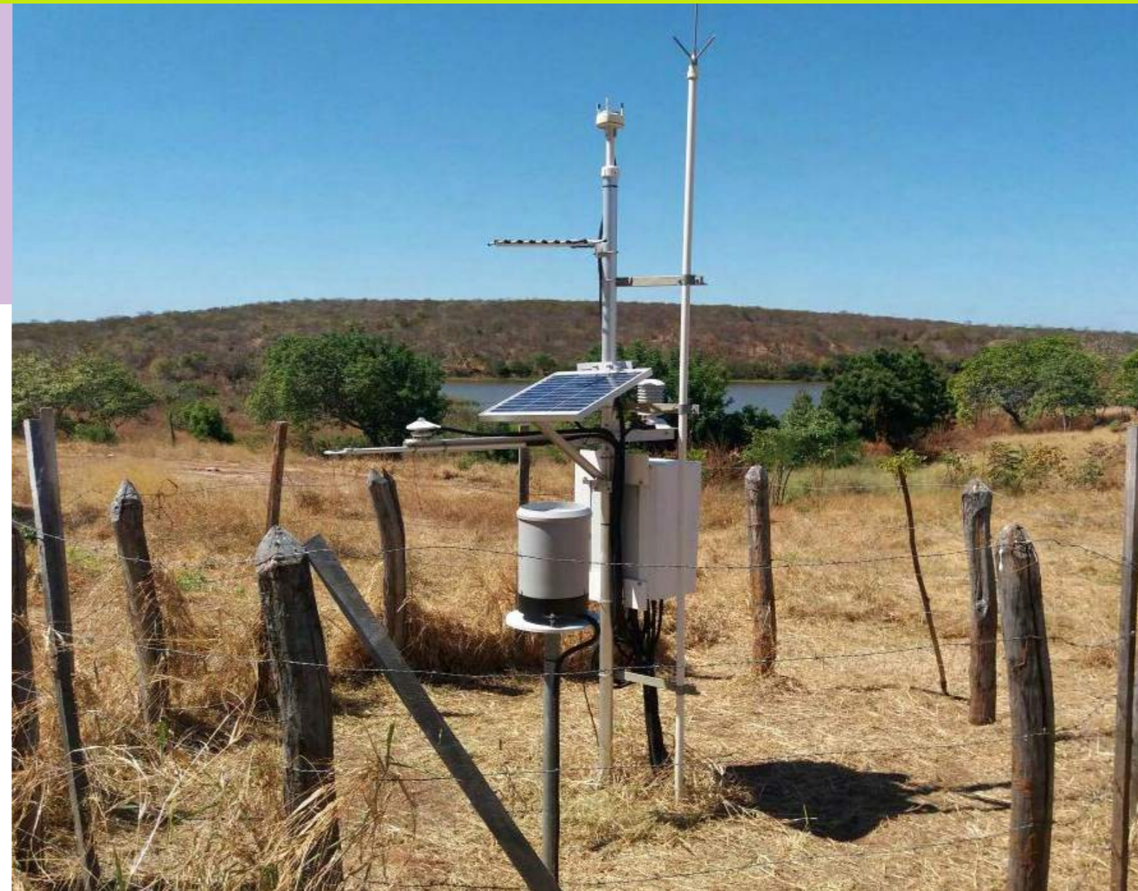
Sensors are used to gather observational data to support drought monitoring in Brazil. Credit: José Maria Costa
