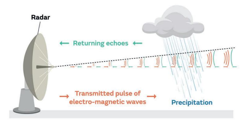
RADAR = RAdio Detection And Ranging
