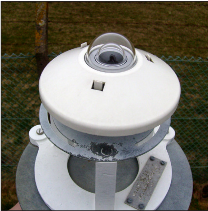
Figure 24. Pyranometer for measuring global radiation.
