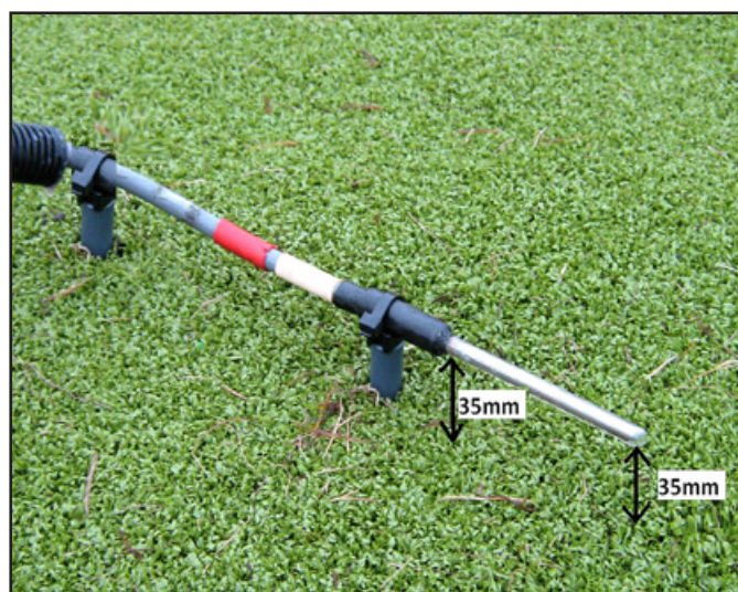
Figure 7. Grass minimum thermometer over an artificial grass surface
