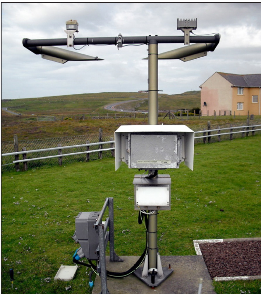
Figure 22. Present weather sensor.
