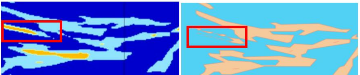
Figure 5. GRIB2 turbulence data on the left, polygon data on the right, which displays dashes as a result of the smoothing resolution along a narrow region of Severity 1 Turbulence (thin band of light blue on the left).
