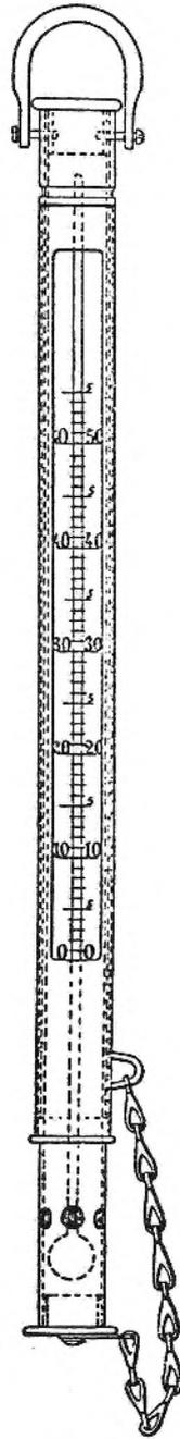
Fig. 2. Thermometer for measuring the water surface temperature. At the bottom on the chain is the sleeve which is opened after observations to let water out of the chamber. The interrupted lines show the position of the thermometer bulb in the metal holder.
