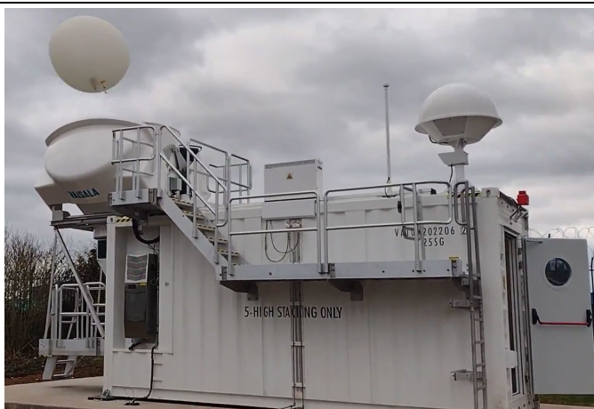
Figure 1. The Vaisala AS41 Autosonde at Nottingham, Watnall releasing a balloon-borne radiosonde.
