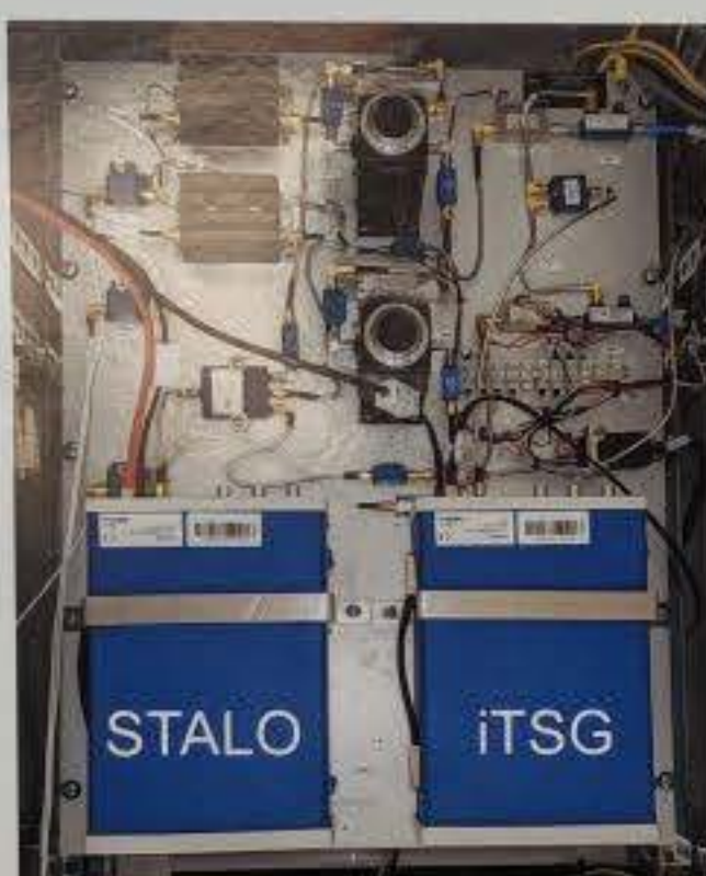
Fig. 1: Radar receiver box with two integrated AnaPico APSIN6G (STALO left, iTSG right). The path to the CGC is not visible.
