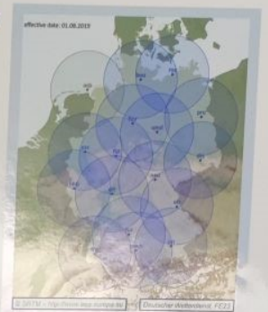
Fig. 1: Operational DWD weather radar network shown with a 150 km coverage radius. Geo data: ©SRM – http://www.eea.europa.eu .
