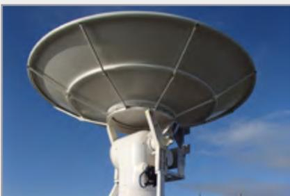
A device that sends out electromagnetic pulses which detect objects in the sky, like raindrops, and can tell how big they are, where they are and how fast they are falling.
