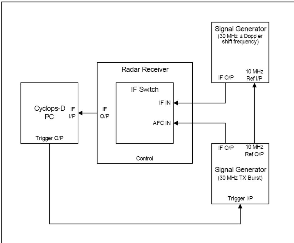
Fig 6. Test harness for the radar receiver and signal processor.
