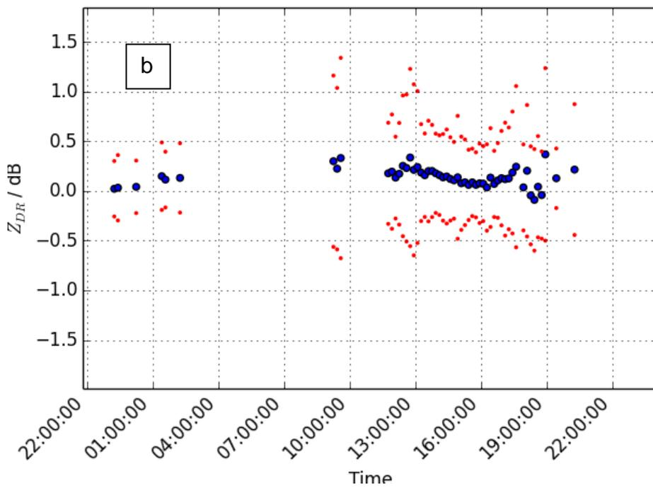
Fig 11. Sample time series of  $Z_{dr}$  offset obtained from measurements at zenith in rain from the Predannack radar. a) shows data from 26 January 2014 – an example of a day with high stability, and b) is from 25 May 2014, which is typical of the largest diurnal variations that have been observed. The larger symbols are the mean values of  $Z_{dr}$  recorded during the scans, and the smaller symbols above and below show the standard deviation.
