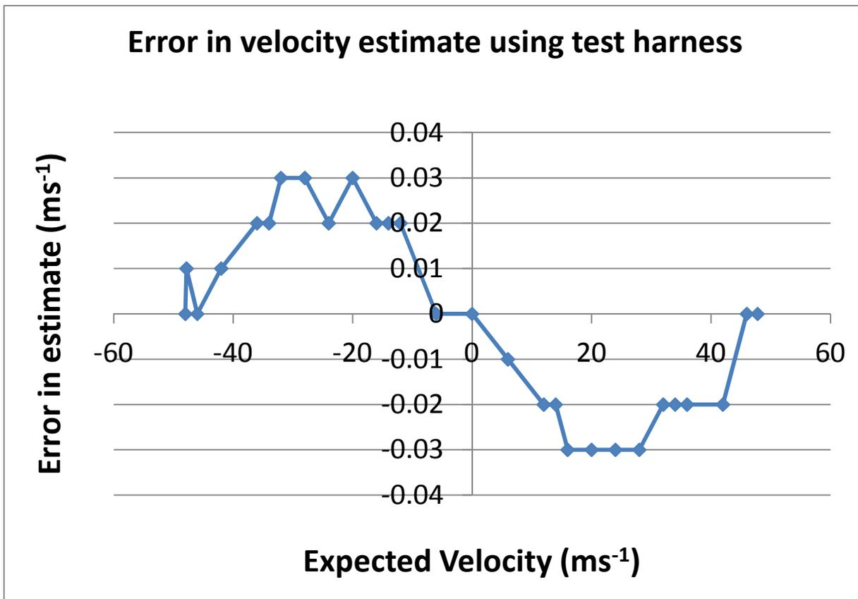
Fig 7. Errors in velocity recorded using the test harness in Fig 6.
