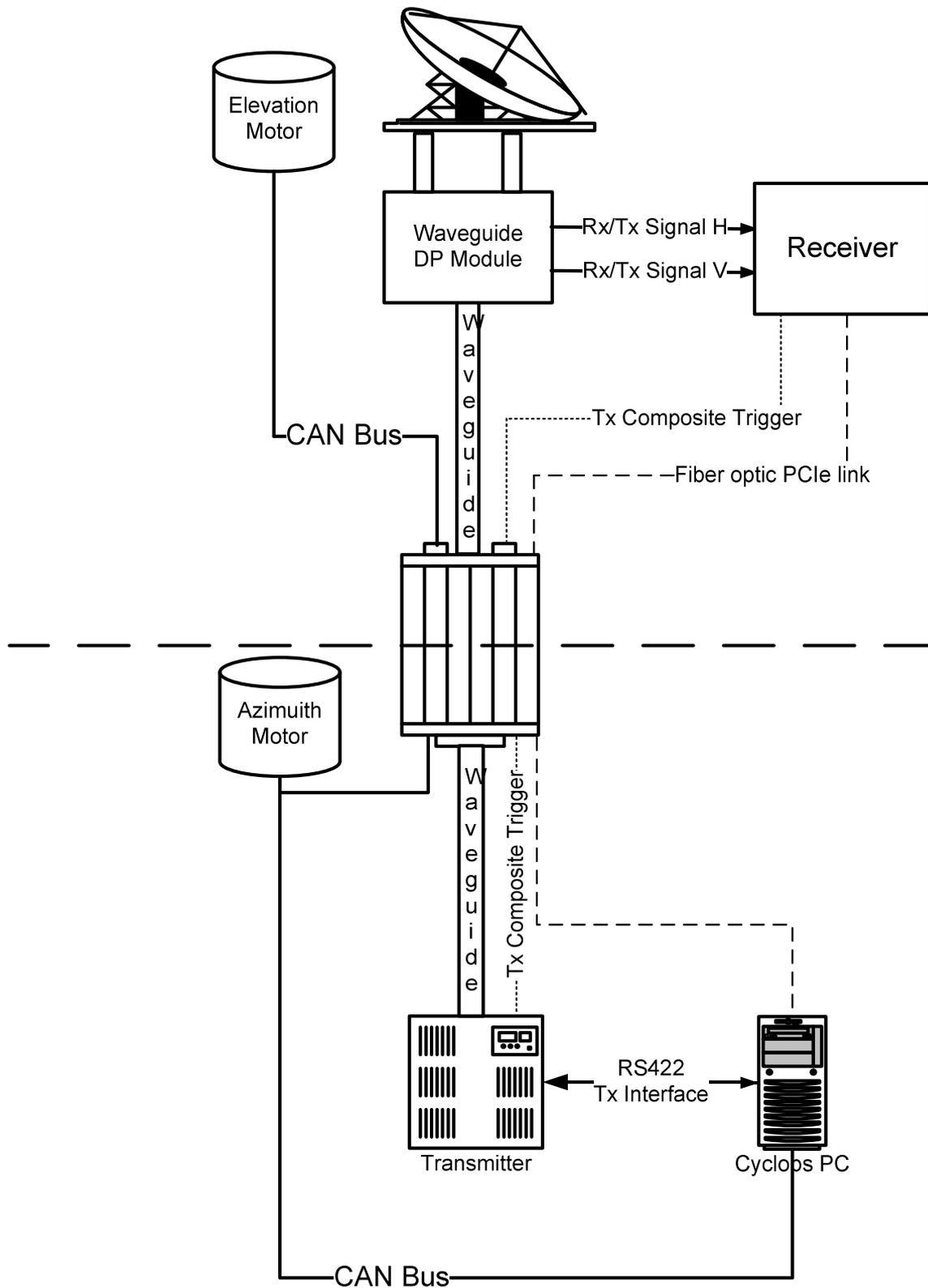
Fig 1. Radar architecture overview. Components above the dashed line rotate in azimuth..
