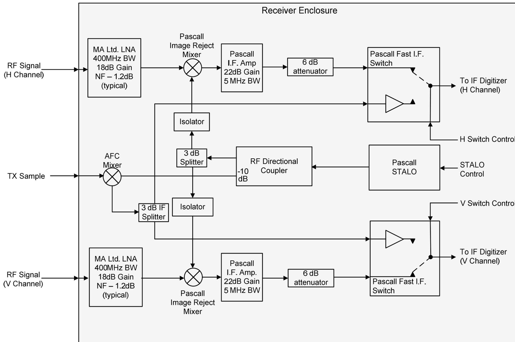
Fig 3. Block diagram of dual-channel receiver
