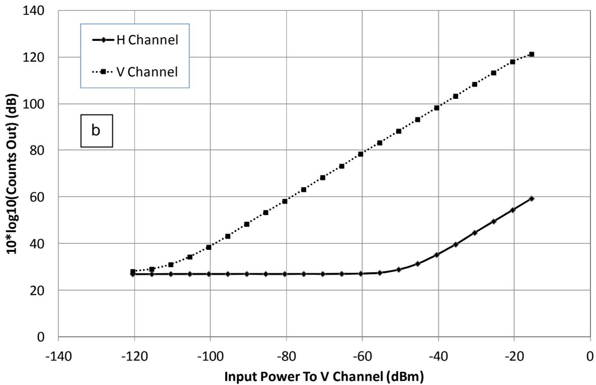
Fig 8. Results from calibration of the dual-channel receiver. a) signal injected in the H Channel and b) the V channel.
