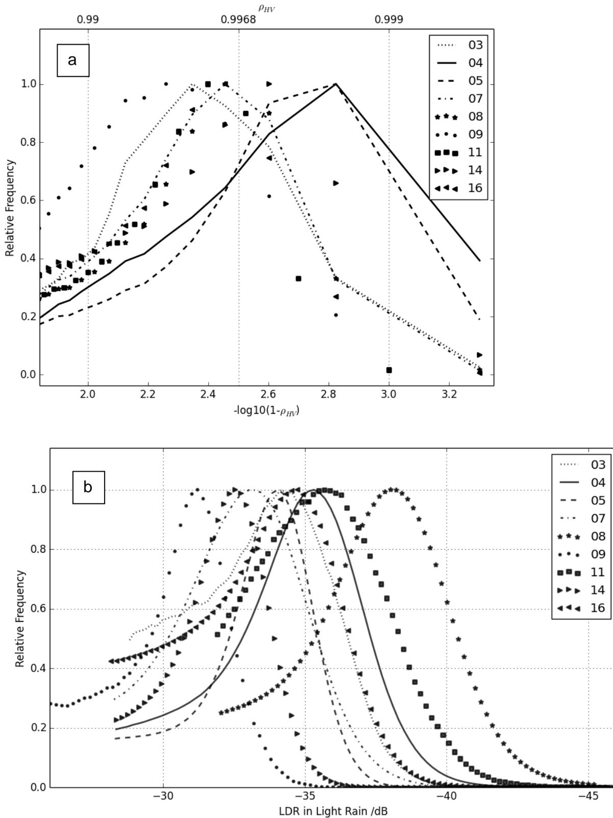
Fig 9. Frequency distributions of a)  $\rho_{HV}$  (transformed to a log scale to aid clarity) and b) LDR recorded in areas of widespread non-attenuating rain (measured reflectivity in the range 20-25dBZ) . Table 2 lists the peak values in each distribution.
