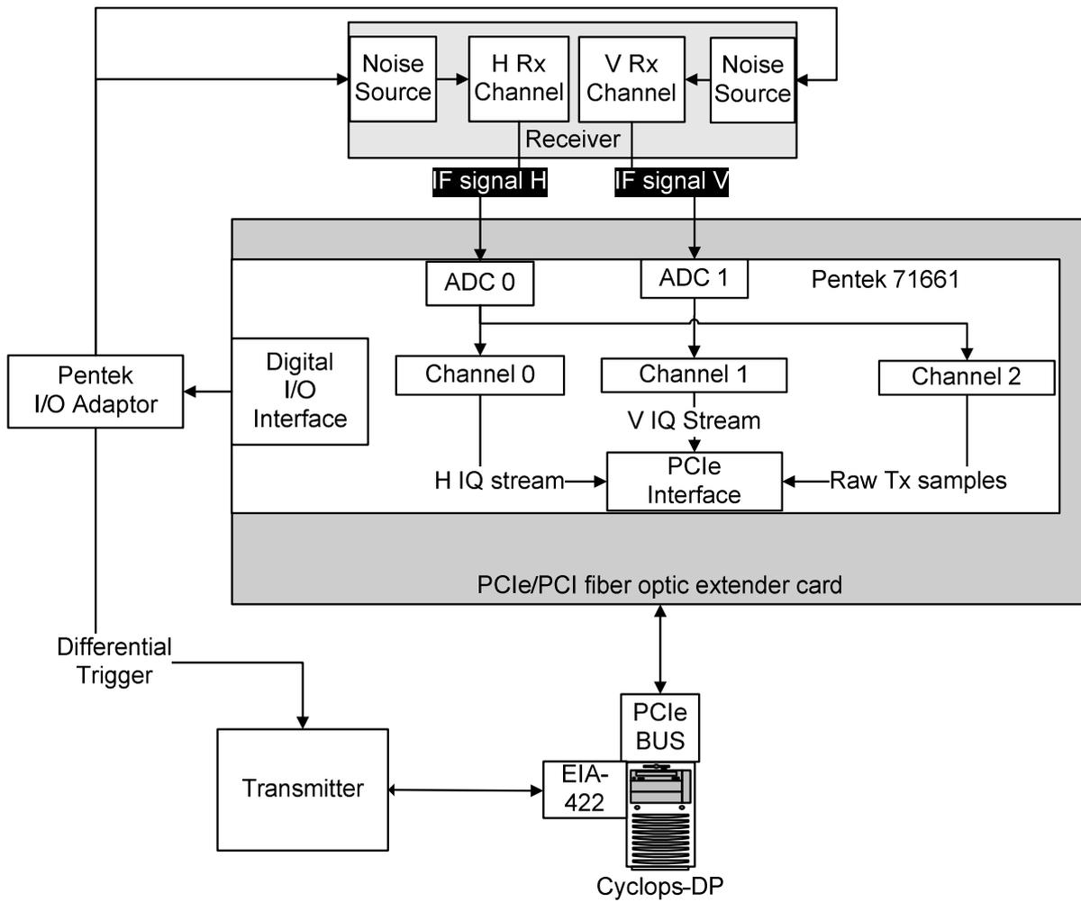
Fig 4. Block diagram of signal processor
