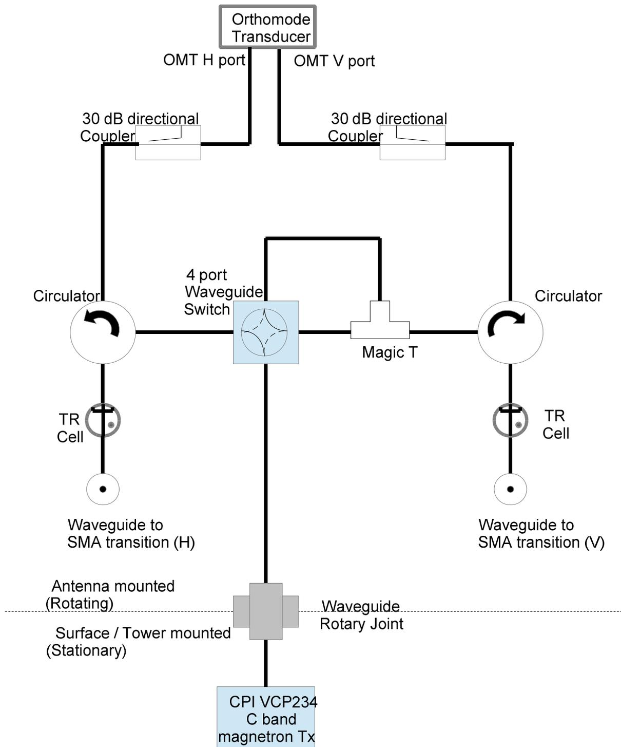
Fig 2. Schematic of waveguide unit located above the elevation axis. The waveguide switch is shown set to the LDR mode of radar operation.
