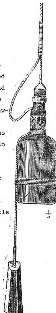
the instrument touch the walls of the glass. The hydrometer is allowed to bob up down a little and then, looking just below the water surface, the precise level on the scale to which the instrument has sunk can be observed.
